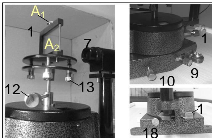
**Figure 4.** Locking, fixing and adjusting screws of the apparatus. A<sub>1</sub>: Fixing screw for the grating; A<sub>2</sub>: The grating. 7, 9, 10, 12-14, 18 and 19 are explained in Figure 2.
