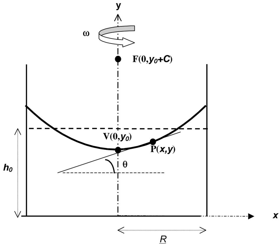
**Figure 1.** Definitions of the bank angle  $\theta$  at point  $P(x, y)$ , the vertex  $V$  and the focus  $F$  for the parabolic surface produced by rotating the liquid, of initial height  $h_0$  and radius  $R$ , at a constant angular speed  $\omega$  around the  $y$ -axis.
